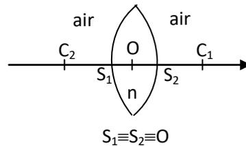
$$R_1 = \overline{S_1 C_1} = R \quad \text{et} \quad R_2 = \overline{S_2 C_2} = -R$$
