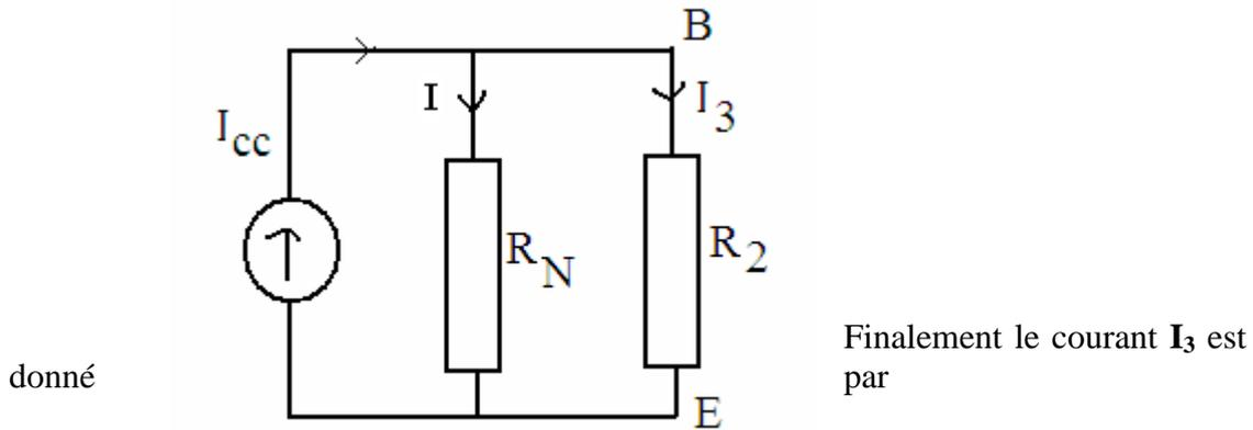
$$\begin{cases} R_N I = R_2 I_3 \\ I + I_3 = I_{cc} \end{cases} \text{ et donc } R_N (I_{cc} - I_3) = R_2 I_3 \Rightarrow I_3 = \frac{R_N I_{cc}}{R_2 + R_N}$$
